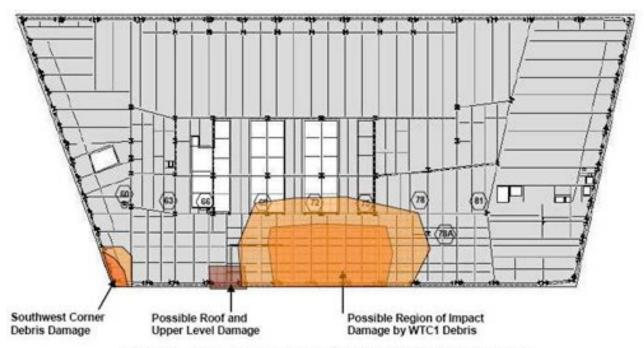
Figure L-23c. Possible extent of debris damage in plan.
